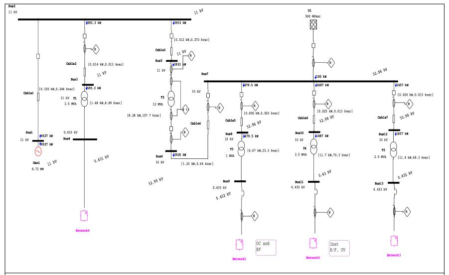
This is a ETAP LOAD FLOW output while the system works on "Captive Generation FLOAT" mode.
