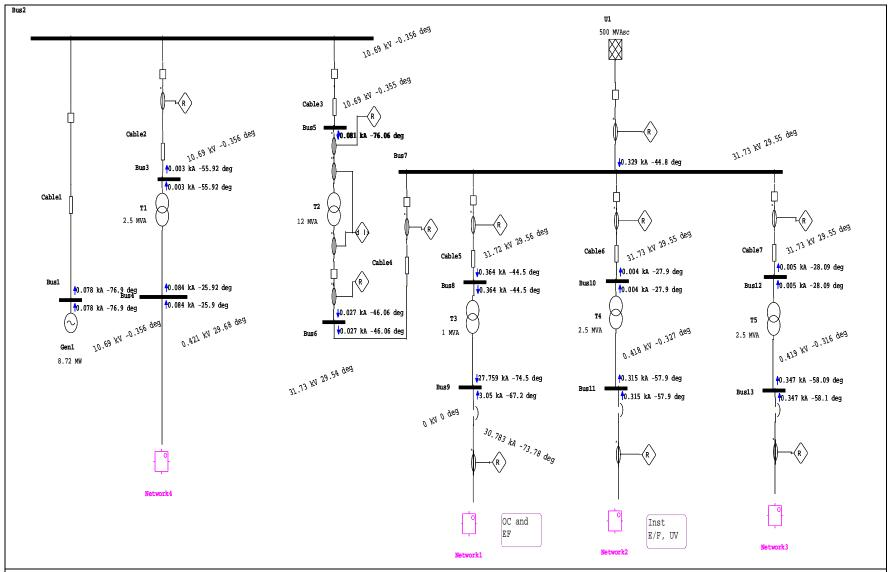
This is a typical SC analysis output from ETAP showing SC fault at Bus 9 - secondary of 1 MVA process load transformer. For eaze of reading – please Zoom this diagram on computer.
