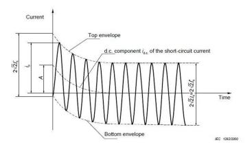
Short circuit is a disturbance in electrical system and usually it starts with **huge** (several times more) asymmetric current having DC component and then after some cycles it settles down to a symmetric value.
