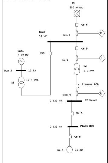
**Zone 1 CB B and A:** These are MCCBs and needs to be coordinated locally for fault isolation based on facilities available on breaker.
