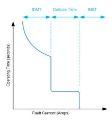
Heat generated due to electric current is proportional to  $I^2$  as such the trip time should reduce in proportion to increase in  $I^2$ .
