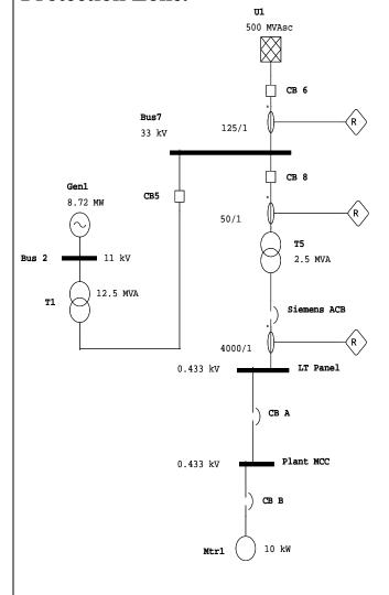
**Zone 1 CB B and A:** These are MCCBs and needs to be coordinated locally for fault isolation based on facilities available on breaker.
