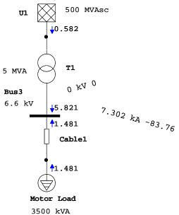
As shown above, if motor loads are involved, then at the time when short circuit happens, the motor acts as generator till they come to stand still and feed to the fault. In above case 7.302 KA is fault current and it comprises of 5.821KA coming from source and 1.418 KA from motor load. Large inertia motor loads can keep feeding the fault, till the fault is cleared and hence need to be considered while designing breaker short circuit capacities.
