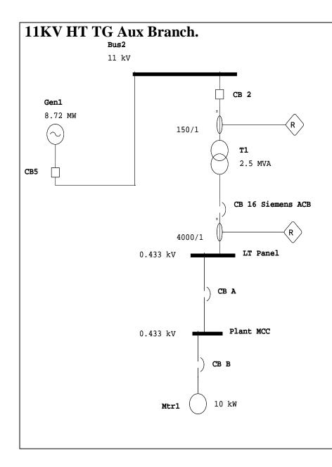
**Zone 1 CB B and A:** These are MCCBs and needs to be coordinated locally for fault isolation based on facilities available on breaker.
